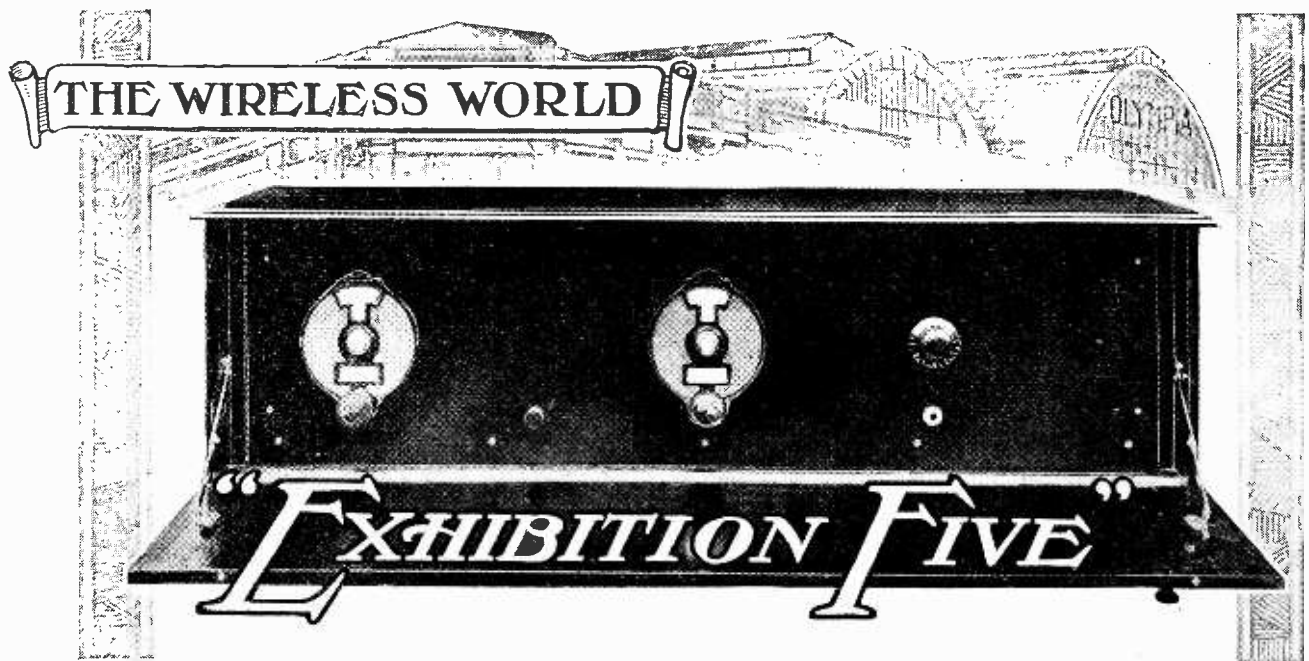
Two Tuned H.F. Stages without Screening or Neutralisation.
