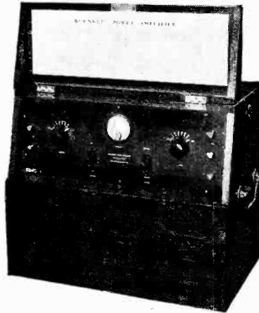
The Burndept Power Amplifier for use in conjunction with Rice-Kellogg and other large Loud-speakers.
