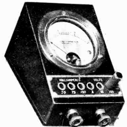
Siemens combined Volt and Milliampere-meter provided with six ranges.
