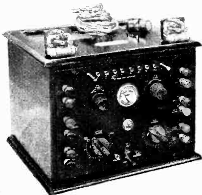
The Ekco Combined Battery Eliminator H.T., L.T. and grid bias for D.C. mains.
