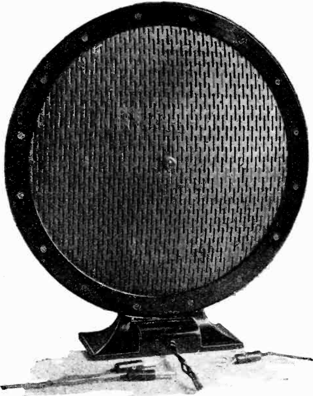
The Vogt electrostatic loud-speaker in which the moving diaphragm consists of an aluminium disc only 0.02mm. in thickness.
